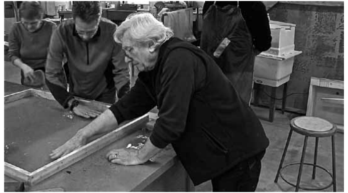
John Babcock gets help from Lois James and Peter Sowiski to sponge the back of his newly poured sheet comprised of pigmented cotton segments without a base sheet.
